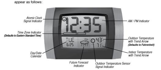
The clock will initially set itself to the correct time and date, defaulting to EST (Eastern Standard Time). It will also begin displaying the temperatures. The clock will begin searching for the Atomic signal.
